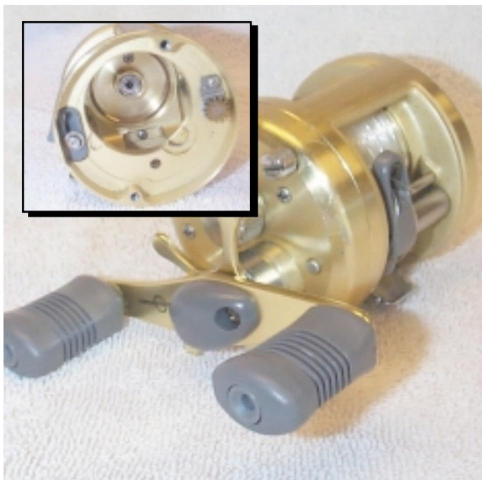
This 6-year-old Shimano CT 250, used in saltwater and treated regularly with CorrosionX, shows no sign of corrosion inside or out.
