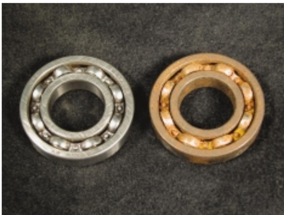
The bearing on the left was treated with CorrosionX; the one on the right was left untreated and both were sprayed with seawater every day for two weeks. Note the remarkable difference.
